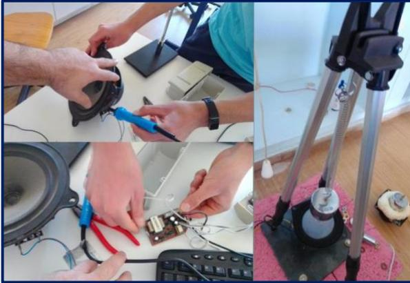
**Figure 6** Images of the construction of a digital seismograph
